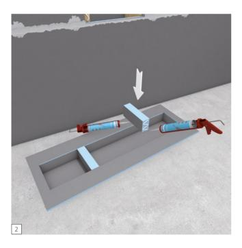
When available, wedi shelve units can be installed by gluing these into the interior of the niche and flush with its front. wedi Joint Sealant or a 100 % silicone may be used to adhere the shelf on all three sides. In addition, all transitional seams from shelf to niche have to be covered with such sealant which must be spread flat over these seams. A pitch in for the shelf will not be necessary due to the small area but may be introduced during tiling through slight pitching of the tiles.
