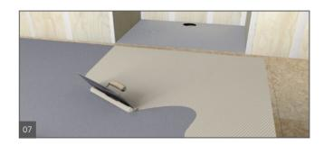
Trowel the thinset on the rear side of the Fundo again using a  $10\times10$  mm notch trowel.
